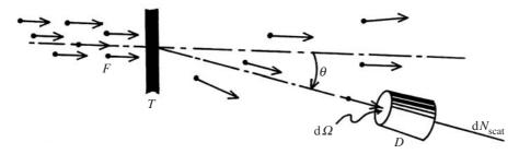
**Figure 5.5** A beam of particles of flux F hitting a target T which scatters some of them into a detector D in the direction  $\theta$ . The detector, which has a sensitive surface  $d\Omega$ , then records  $dN_{\text{scat}}$  scattered particles
